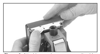
Figure 3. Attaching sandpaper on opposite side.
